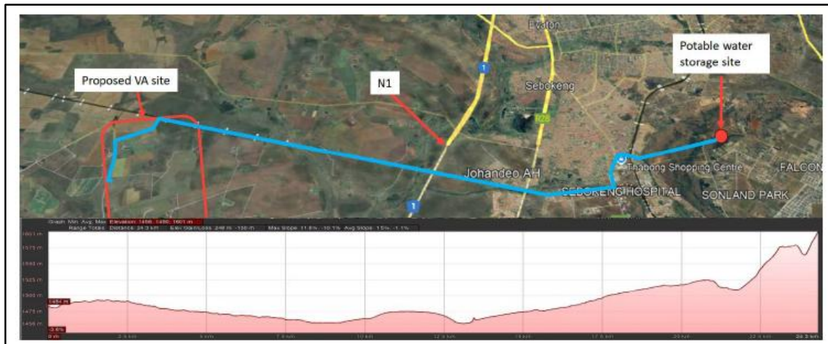
Figure 15: Proposed Rand Water Pipeline Route
