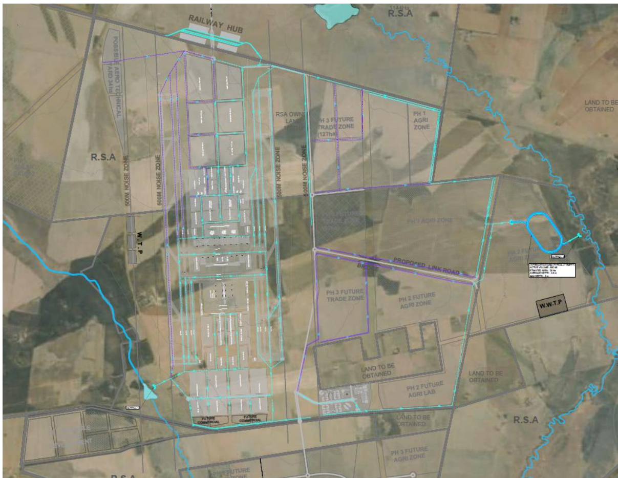
Figure 20: Major Stormwater Routes
