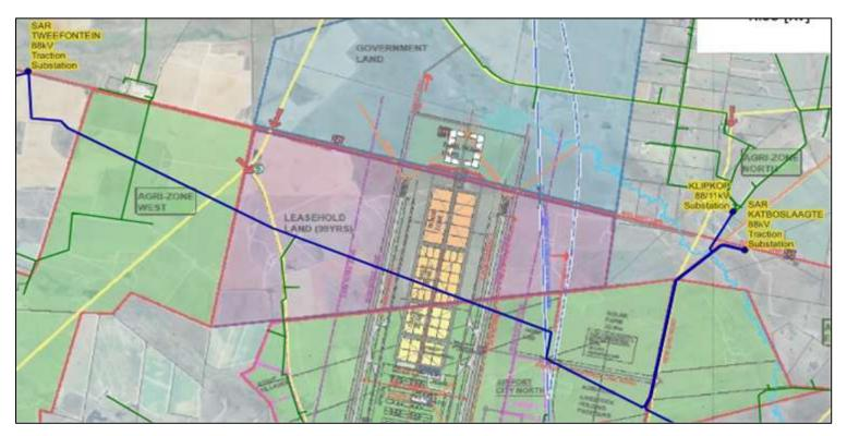
Figure 8-9. Existing 88kV Overhead powerline.
