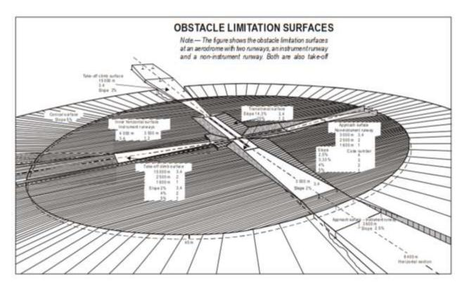
Figure 4-2. ICAO Obstacle Limitation Surfaces (Source: ICAO).
