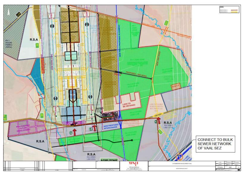
Figure 8-6. Bulk Sewer layout for the First Build.
