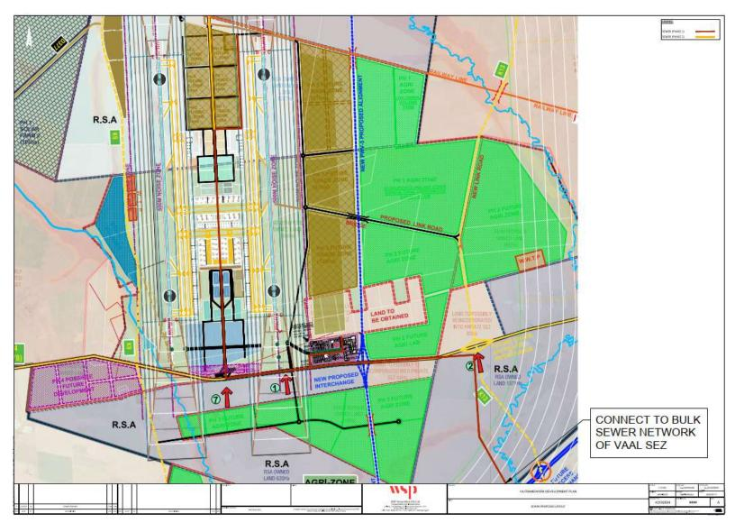
Figure 8-5. Bulk Sewer layout for the ultimate development.
