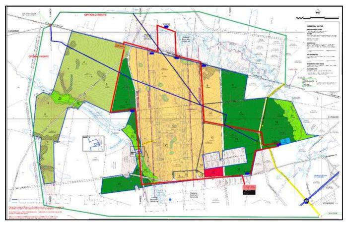
Figure 8-10. Proposed relocation of overhead line and servitude.
