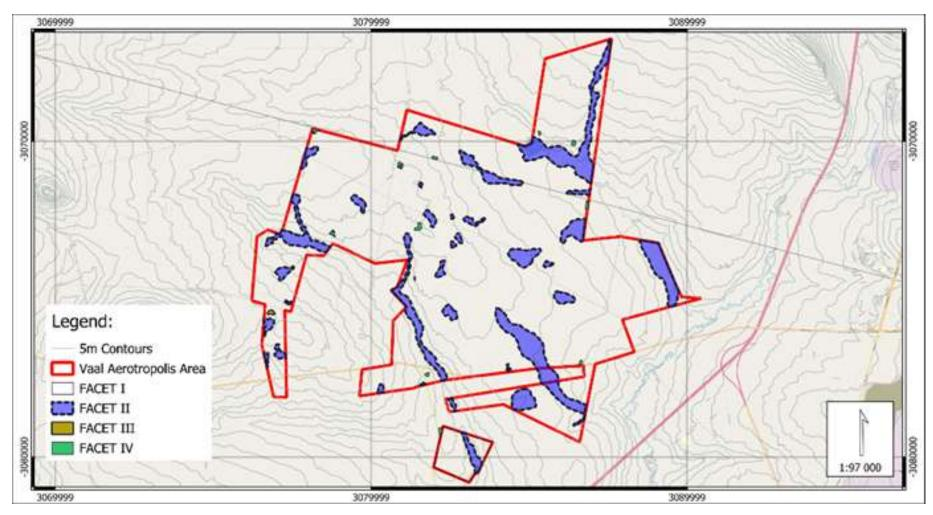
Figure 4-18. Simplified FACET areas of similar geotechnical constraints.
