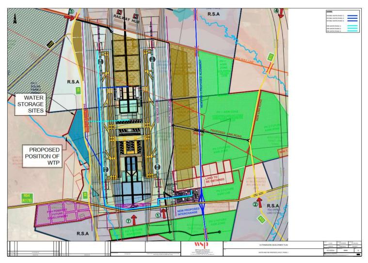
Figure 8-4. Water and Fire supply layout for phase 1.
